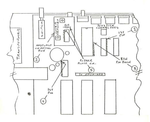
After approximately October 1984, Radio Shack introduced another revision of the COCO II. This version is identified by Model #26-3134A or #26-3136A. If you have one of these, connect your U.V.D. as shown at the left and peoceed to the checkout section of the regular instructions.
