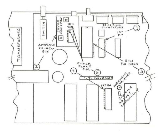
After approximately June 1984, Radio Shack introduced a revised version of the COCO II. This new version is identified by Model #26-3134, or #26-3136. If you have one of these newer models, connect your U.V.D. as shown at the left. Mount the U.V.D. on top of the joystick connectors. Lift the keyboard out of the way to connect the black audio clip #5. Proceed to the checkout section of the regular instructions.
